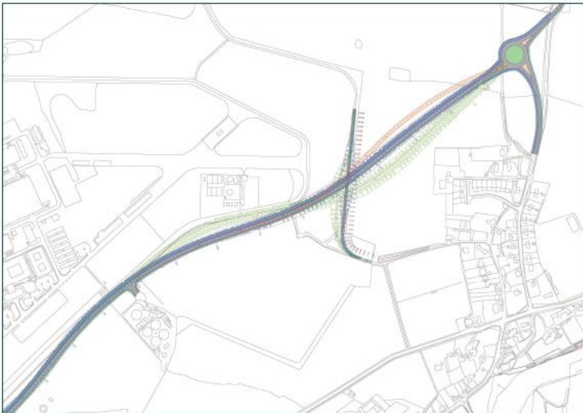
Plan showing alignment options considered for Clifton Hampden Bypass
